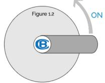
For wall lever taps we recommend this way for installing them as if the gland nut is loose (needing re-tensioning) gravity will push the tap to a close.
