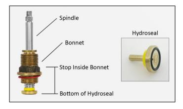
The turn of the mechanism is guided by the distance between a stop machined inside the bonnet and the bottom of the Hydroseal tap washer. Our mechanism has a quick rise thread so it rises open in a shorter distance than a standard tap spindle. Approx 0.6mm of length of thread gives ¼ of a turn of movement.
