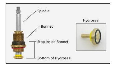
The turn of the mechanism is guided by the distance between a stop machined inside the bonnet and the bottom of the Hydroseal tap washer. Our mechanism has a quick rise thread so it rises open in a shorter distance than a standard tap spindle. Approx 0.6mm of length of thread gives ¼ of a turn of movement.
