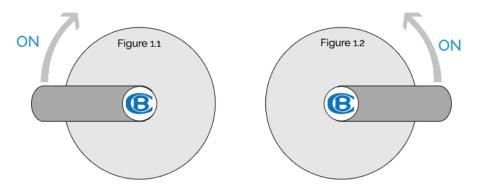
For wall lever taps we recommend this way for installing them as if the gland nut is loose (needing re-tensioning) gravity will push the tap to a close.
