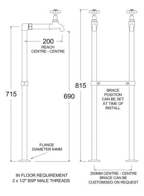
**IMPORTANT:** Maximum hot water temperature 65°C and 500 kPa Maximum operating pressure at any outlet within a building (Ref AS/NZS 3500)
